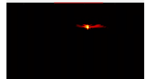
Phase error due to defective carrier frequency
